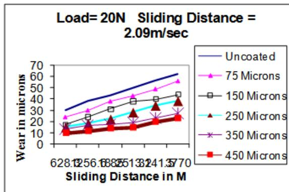
Fig 3: (a, b and c) Variation of Wear with Sliding Distance for a given sliding velocity
