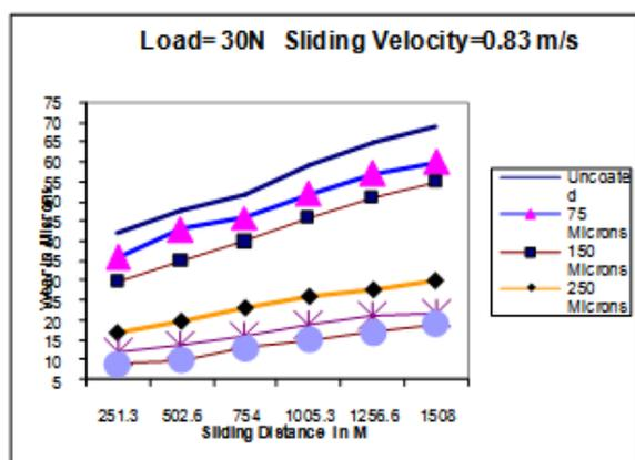
Fig-2 (a, b and c) Variation of Wear with Sliding Distance for a Given Load
