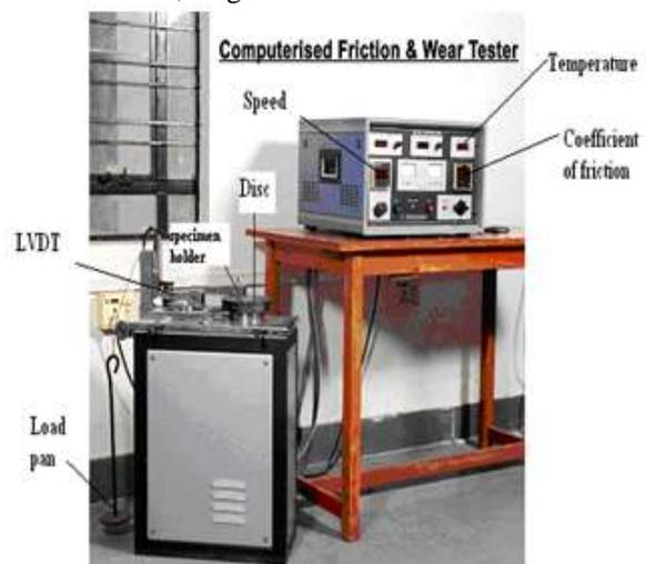
Fig-1 Pin on disc wear tester
