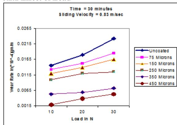
Fig 5: Variation of Wear Rate with Load
